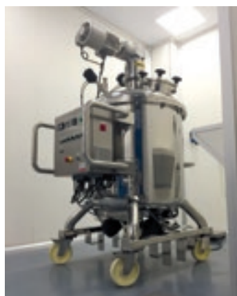
Mobile reactor with slow agitation prepared to work under vacuum and pressure, with electrical control panel attached to the equipment. Outside finishing mirror polished.
