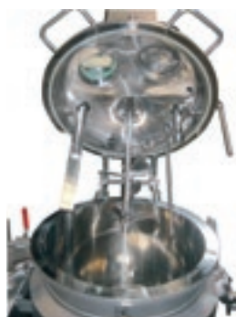
Internal view of diluter designed for vacuum operation
