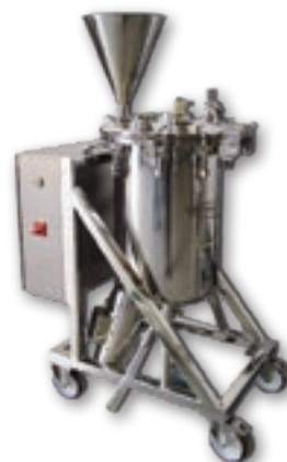
50 Litres reactor with magnetic agitation mounted in the lowest part
